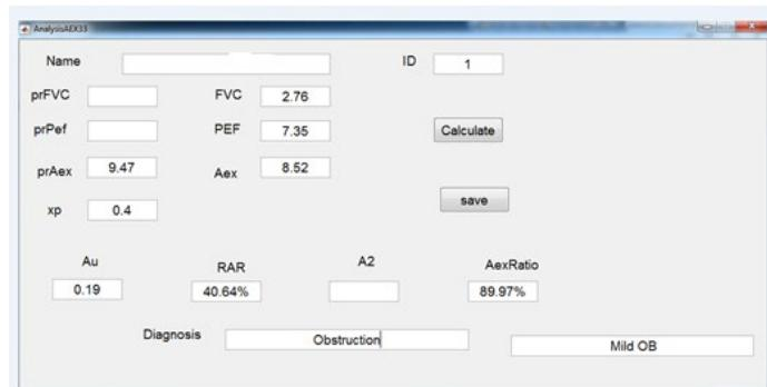
**Figure (1):** The graphical interface in the proposed technique. FVC, forced vital capacity; PEF, peak expiratory flow; Aex, surface area under the maximum expiratory flow volume curve; prAex, predicted Aex; Xp, denotes the expired volume at PEF; Au, denotes the area of concavity below an imaginary diagonal line and above the maximum expiratory flow volume curve; RAR, rectangular area ratio; Aex ratio, measured/predicted Aex.
